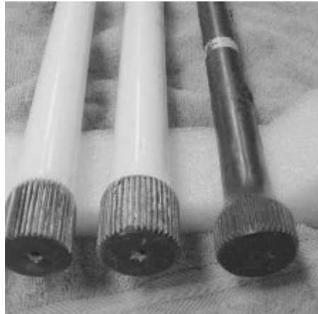
Figure 2 – Splines on the end of torsion bars.
