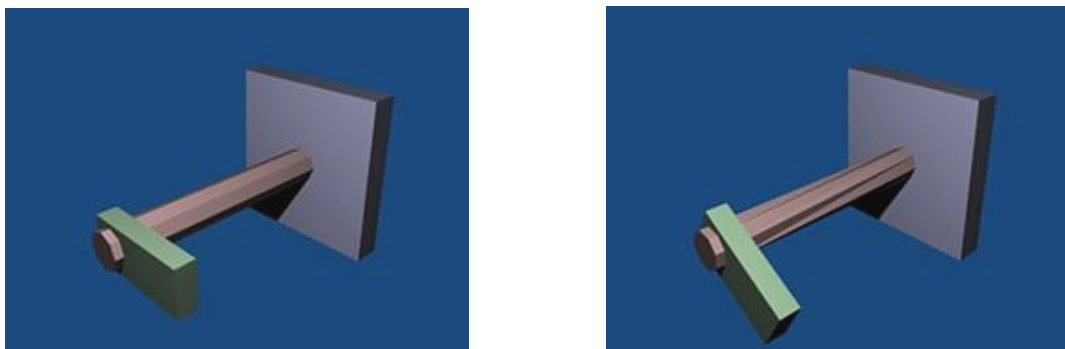
Figure 4 – A torsion bar undergoing twisting.
